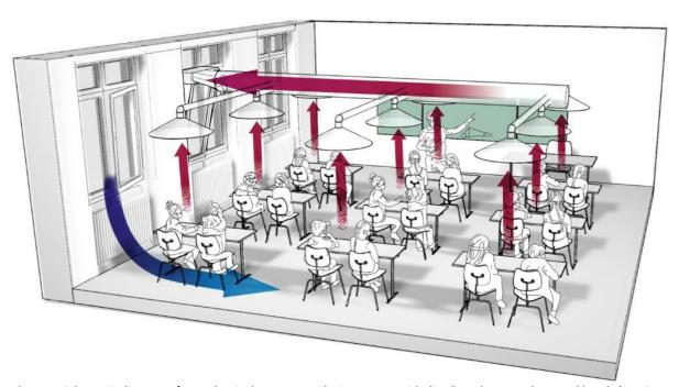
**Figure 4:** Schematic diagram of a mechanical extract ventilation system with distributed extract ducts and hoods (MPIC-MEV hood version) (ventilation-mainz.de).
