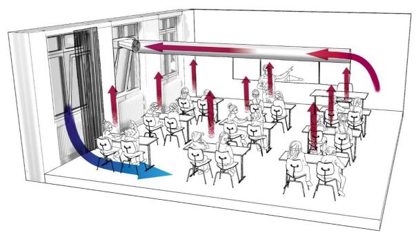
**Figure 3**: Schematic diagram of a mechanical extract ventilation system with central extract duct (MPIC-MEV base version) (ventilation-mainz.de).
