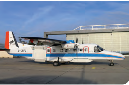
DLR's F-SAR sensor on the Dornier DO 228 carrier platform: The antenna system is mounted at the rear of the aircraft. Image credit: DLR.
