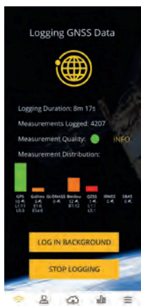
Screenshot from the Camalot Android app that allows users to collect and share raw GNSS data.
