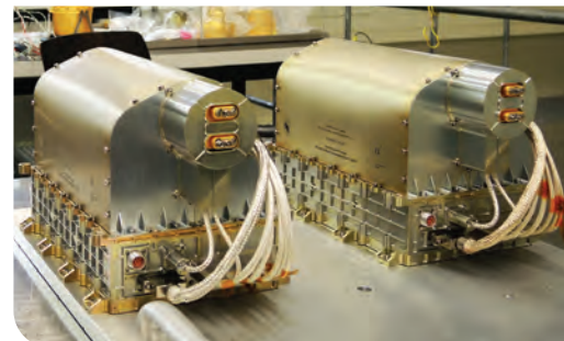
NGMS proto-flight instrument (left) and flight-spare (right) in cleanroom at UNIBE ready for delivery to Roskosmos.
