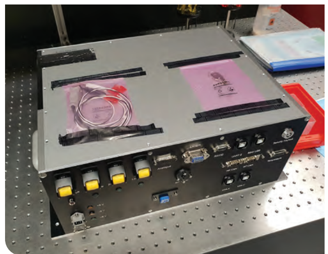
Above: laser box to be used for ground performance and functional tests of the laser pointing system bread-board (Image credit: THALES). Right: assembled control electronics to drive the mechanism movement during ground testing (Image credit: THALES).
