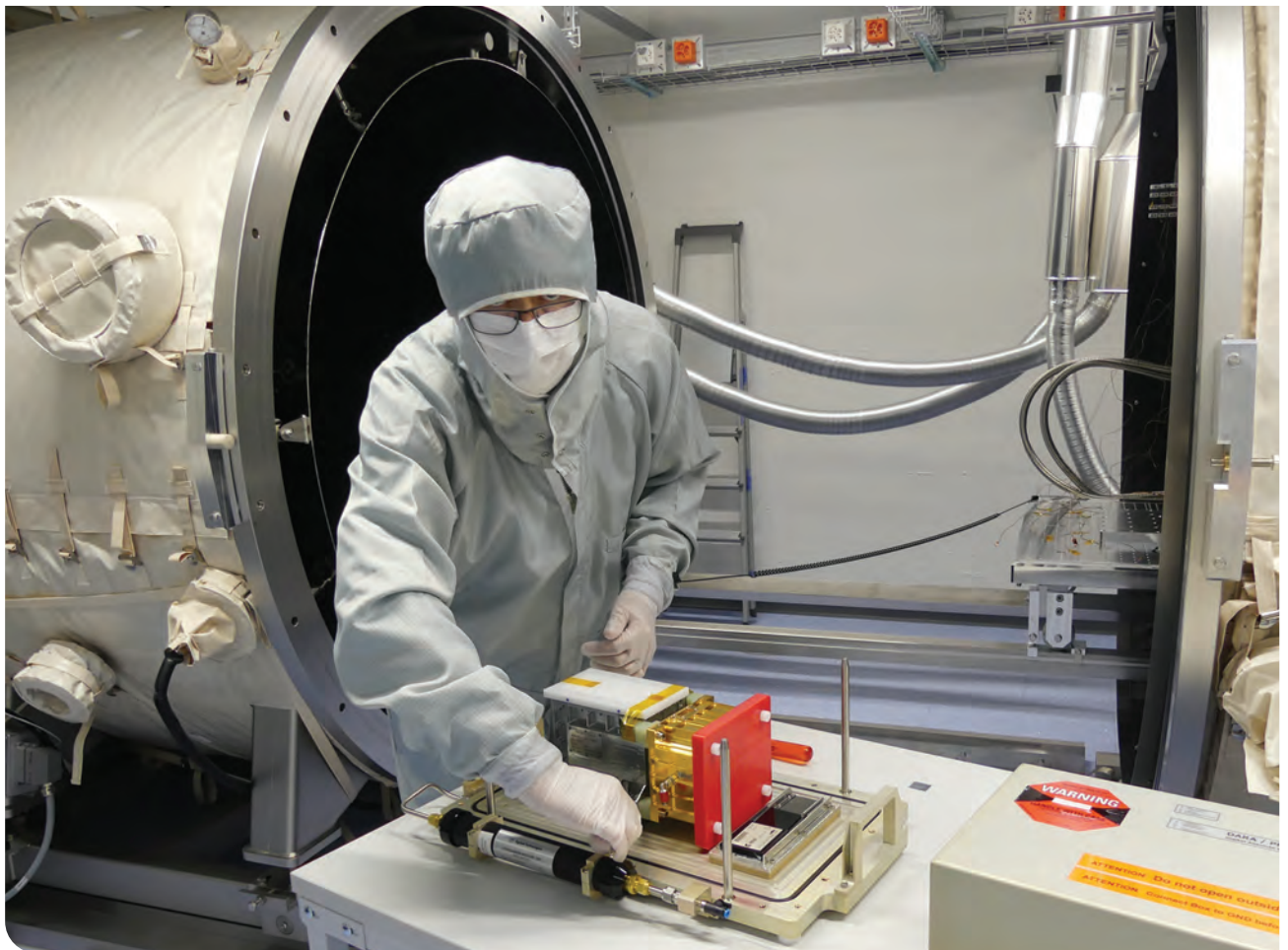
A PMOD/WRC staff member is preparing the DARA FM for thermal-vacuum tests at the University of Bern.
