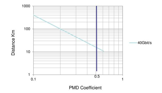
Typical PMD(max) for 40Gbit/s transponder = 2ps. PMD coefficient =0.5ps/ $\sqrt{Km}$ , Max distance is 16Km PMD(max) = 0.5x  $\sqrt{16}$  = 2ps. PMD considered Maxwellian, NRZ coding, 1db power penalty
