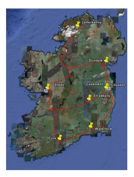
1300Km fiber wrapped on overhead power lines.Combination of different Pylon infrastructure.400Kv, 220KV and 110KVFiber is wrapped and not OPGWSupplier AFL, and the fibre used was corning smf-28.
