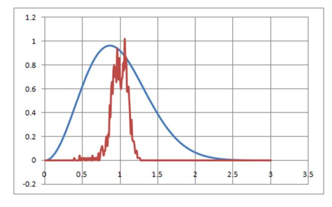
1023 measurements over 3 weeks MEAN DGD 0.974ps PMDq = 0.111ps/ $\sqrt{Km}$ Data sheet PMDq (Link design value 0.1ps/ $\sqrt{Km}$
