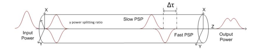
•Asymmetry in the refractive index causes a delay between the Principal states of polarization (PSP) DGD.
