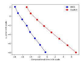
Fig. 4: Efficiency curve of IMEX and explicit time marching schemes for Test 2.
