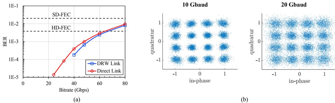
Fig. 4. BER versus the bitrate for 16-QAM-OFDM modulation format and (b) constellation diagrams for recovered symbols.
