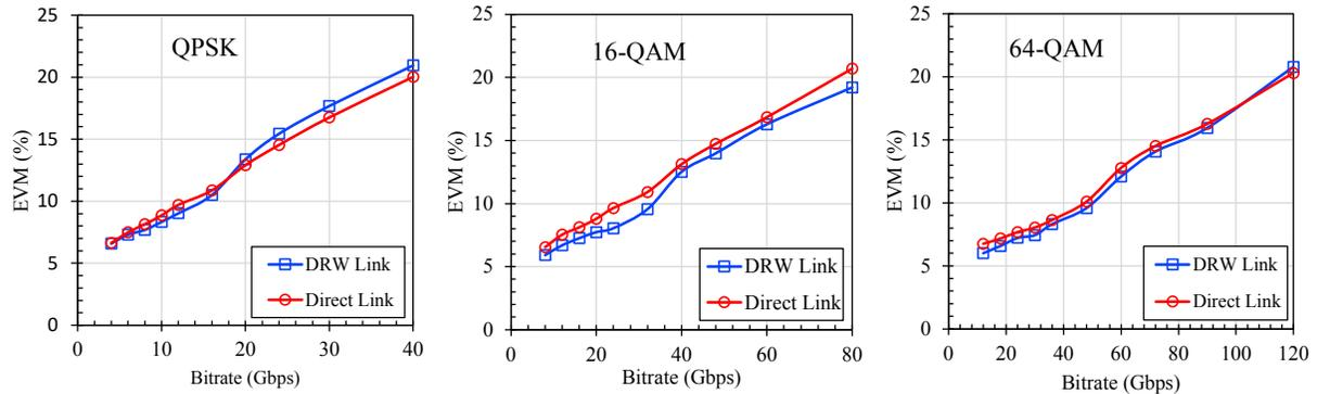
Fig. 3. Measured EVM for THz data transmission for the DRW-based and direct (back-to-back) links at different complex modulation formats of QPSK-OFDM, 16-QAM-OFDM and 64-QAM-OFDM.
