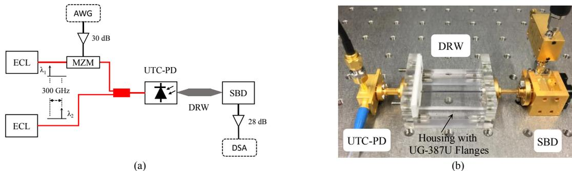
Fig. 2. (a) Schematic diagram of the experimental arrangement used for realising a THz data link at 300 GHz over a dielectric rod waveguide using complex modulation and (b) a photograph showing the DRW assembly mounted on a WR-3 band UTC photodiode and Schottky diode detector.
