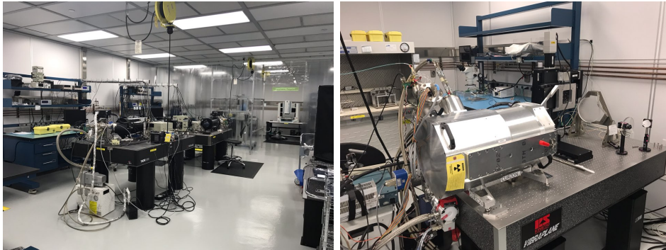
Figure 15: Cleanroom at BNL. Left: Two identical test stands in the picture are TS3-1 and TS3-2. Right: The picture shows TS5 measuring the flatness of nine sensors combined in a raft.
