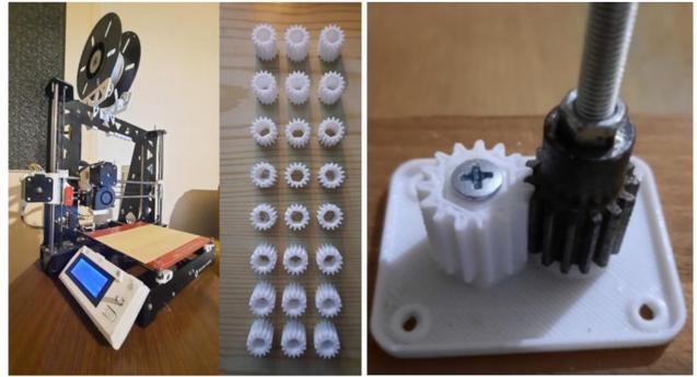
Figure 2:- 3D printer, test gears and testing rig
