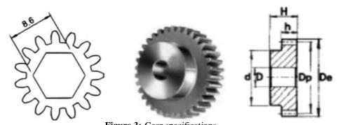
**Figure 3:-**Gear specifications. Modulus m=1 mm, Z=15, h=15 mm, H=25 mm, De=17 mm, Dp=15 mm, d=12 mm, D=6 mm
