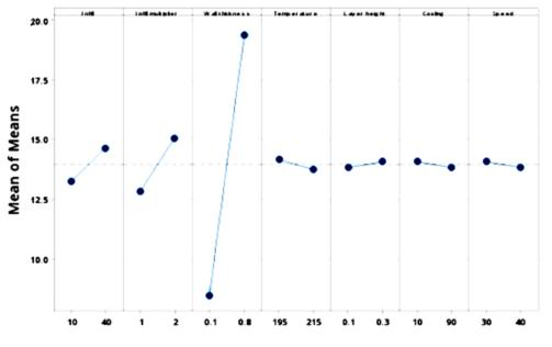
Figure 4:- Main effects plot for means.
