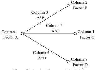
**Figure 5:-** Standard linear graph for  $L_8(2^7)$
