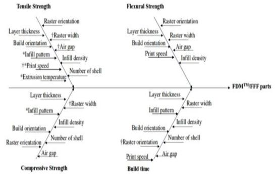
Figure 1:- Diagram of influencing parameters (factors) on the 3D printing process [1].
