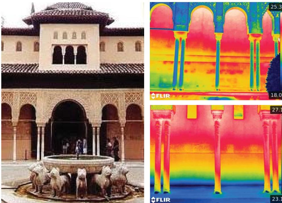
**Figure 1:** General view of Courtyard of the Lions in the Alhambra in Granada (Spain) and images of thermographic measurements. (Source: M<sup>a</sup> Paz Sáez-Pérez)
