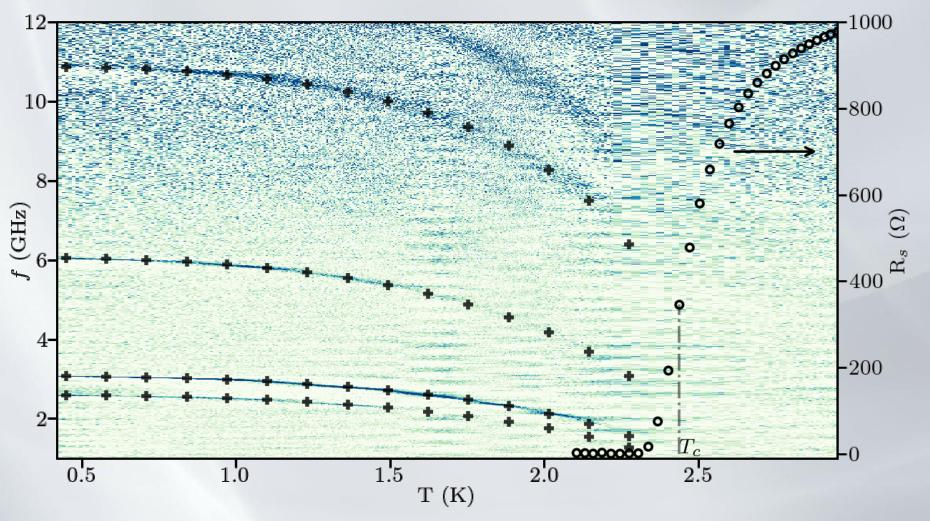
• Resonances in transmission spectra, up to T<sub>c</sub>
