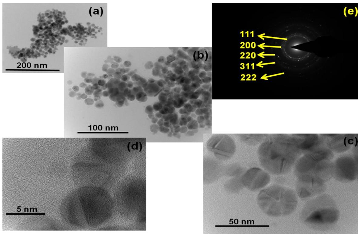
Fig. 2: TEM images (a, b, c, d) of as prepared Ag NPs under different resolutions and (e) SAEDP of crystalline ring structure
