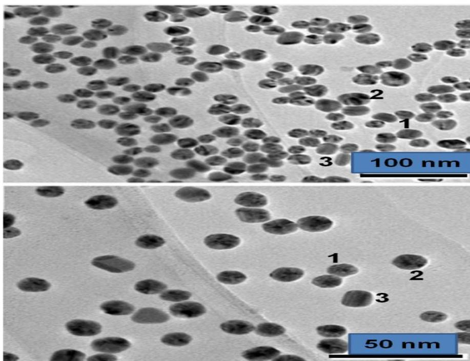
Fig. 3: TEM image of Ag NPs under 100 nm and 50 nm resolution with particles marked 1, 2 and 3 for uncertainty measurements
