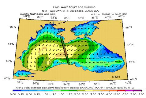
Fig. 5. Collection of altimeter satellite tracks over the Black sea for 17.01.2021 and wave field from WW3 in the Black Sea (the arrows indicate the mean wave directions), the black line denotes the ground track of Altika above the Black Sea on 17.01.2021 at 03h06min (down)
