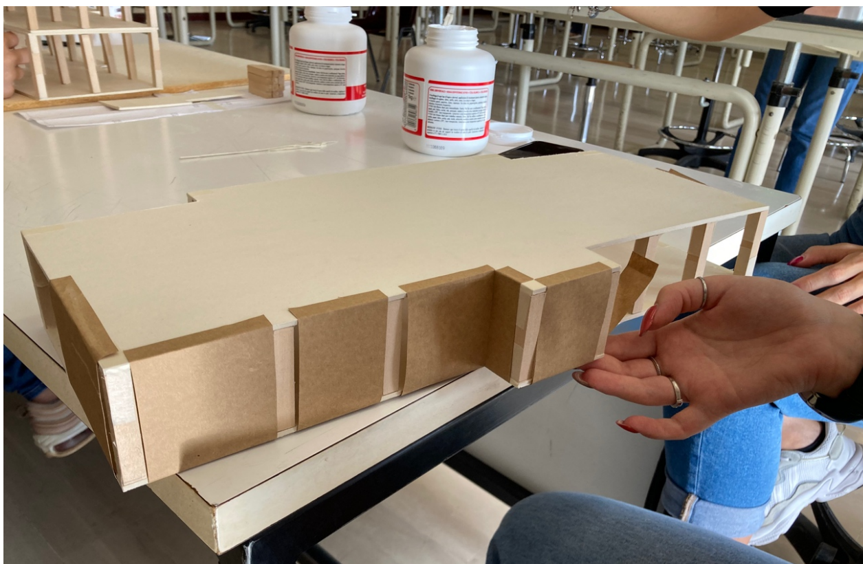
Figure 16: The wall system was simulated by paper rectangles of size mm 50 x 60 glued between the floor and ceiling slabs.
