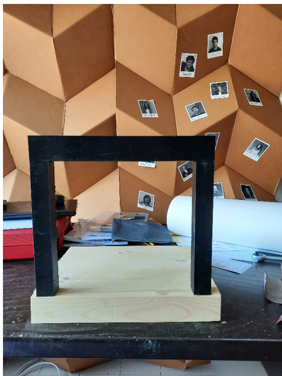
Figure 24a: First one-storey one-bay planar frame.
