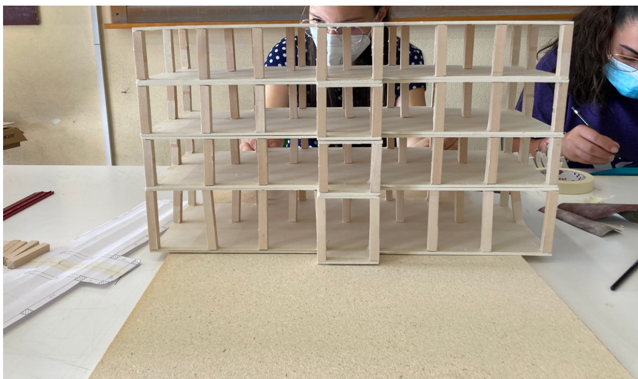
Figure 15: The modules, simulation of the five pilot floors, constitute the base of the structural model on which the interchangeable parts apply: the walls and the panels of the e-SAFE system.
