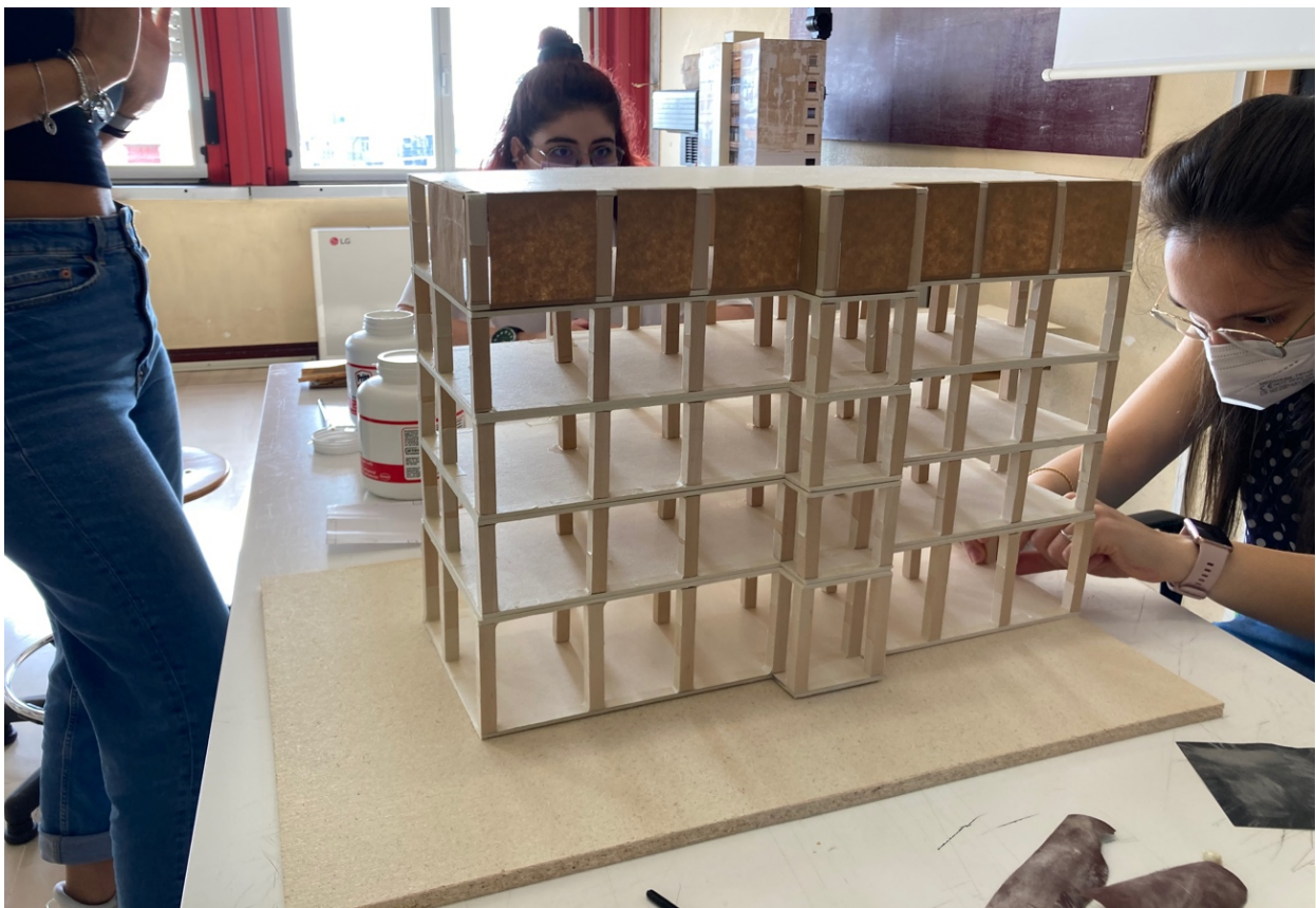
Figure 21: The assembly phases of the structural model.
