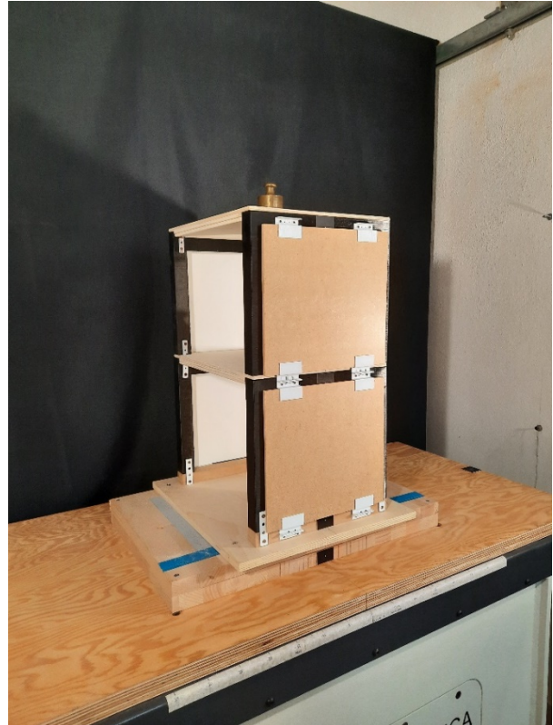
Figure 26b: The final model equipped with e-CLT panels
