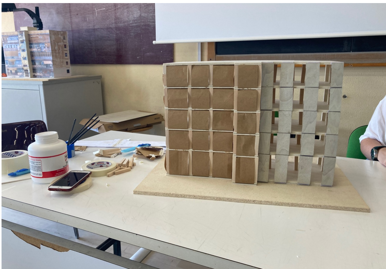
Figure 19: The e-SAFE technology was simulated using 25 x 60 mm plywood rectangles. One part of the structural model was covered with paper rectangles, the other with plywood.
