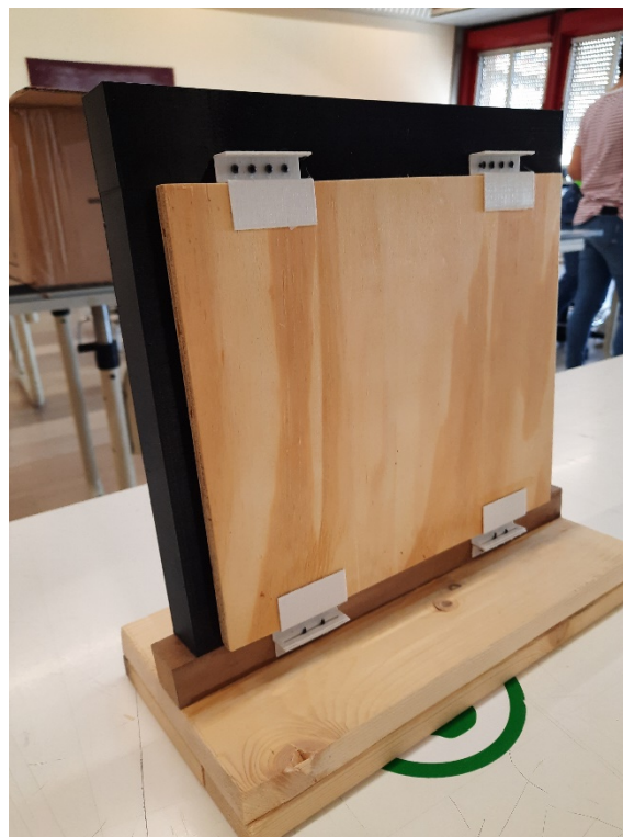
Figure 25b: First step of the model equipped with the e-CLT panel.
