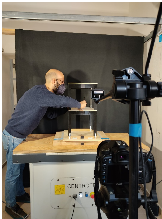
Figure 28: The RC frame model placed on the vibrating table.
