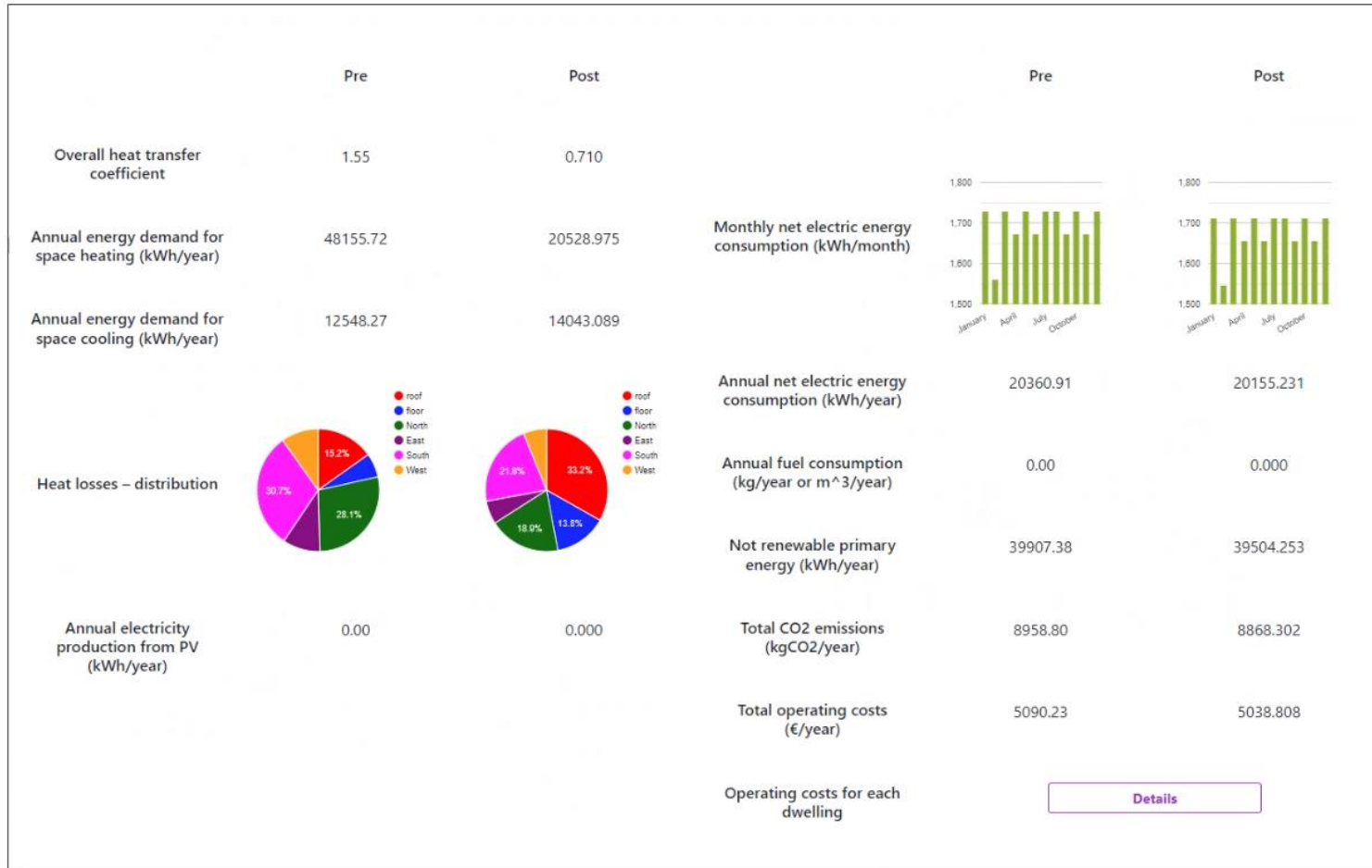
Figure 21: comparison between the pre and post renovation performance -2
