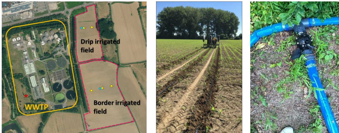
Figure 13: Overview of demo site (left), drip irrigation system installation (center), electro-valve regulating irrigation in each sector (right).
