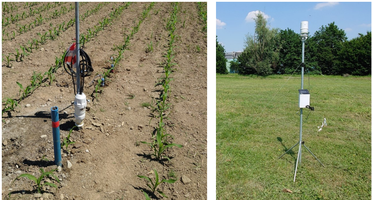
Figure 14: Sensors and devices installed: piezometer, water content probe + GSM modem, porous cups (left); agrometeorological weather station (right).
