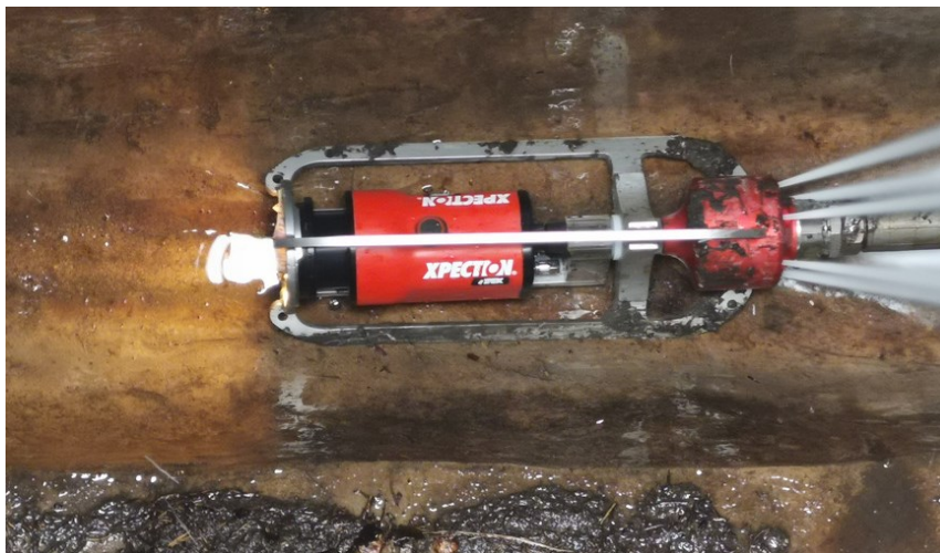
Figure 15: A iPEK XPECTION device for smart sewer cleaning.
