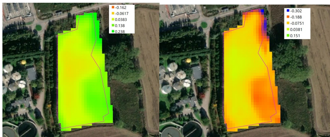
Figure 24: Left: evaluation of the SLWS (20 th Jul 2021); green pixels are related to areas with lower stress; purple refers to areas with higher stress. Right: evaluation of the SLNS (20 th Jul 2021); green-orange pixels are related to areas with lower stress; dark orange /purple refers to areas with higher stress
