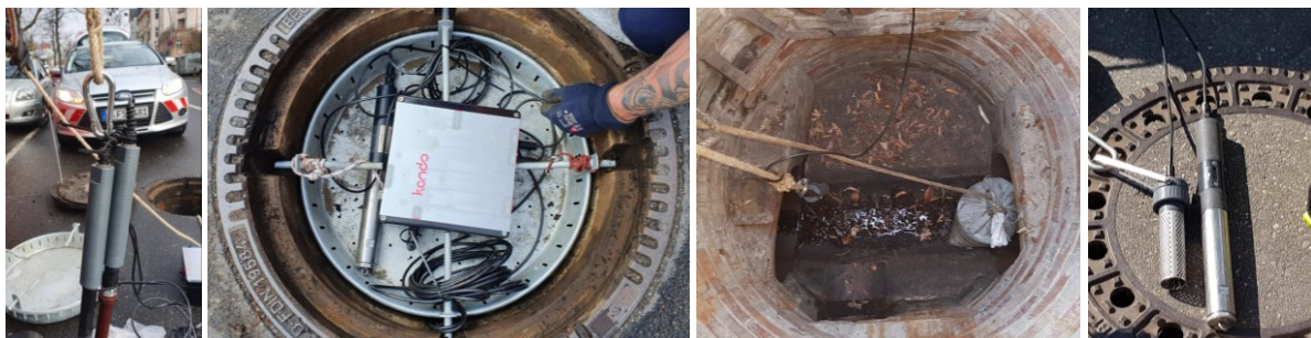
Figure 6: KANDO's smart unit and sensor (left), the EC sensor and logger (right) as well a sensor installed at a sewer manhole (right).
