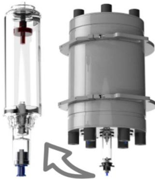
Figure 3: The ALERT V2 instrument, including a zoom on the sampling cartridge, at left. The cartridges are inserted in the instrument from the bottom, their sampling check valves being immersed in the water body of interest. Regarding the cartridge, from top to bottom we can identify the vacuum sampling port and hydrophobic filter, the transparent reaction chamber, the diffuser and isolation check valve, the reagent chamber and the sampling check valve.
