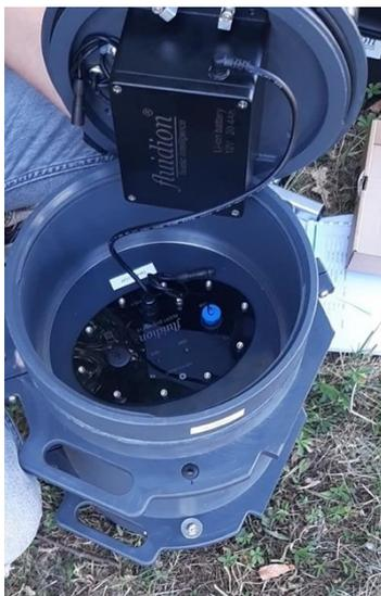
Figure 37: battery replacement
