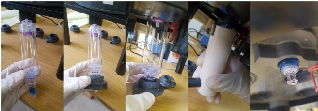
Figure 29: Maintenance of the ALERT System V2; Replacement of the sample cartridges.
