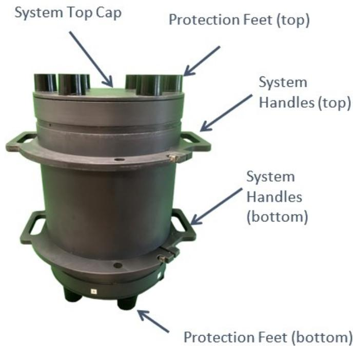
Figure 5: The external mechanical details of the ALERT V2 instrument. The sampling ports are located at the bottom of the instrument.
