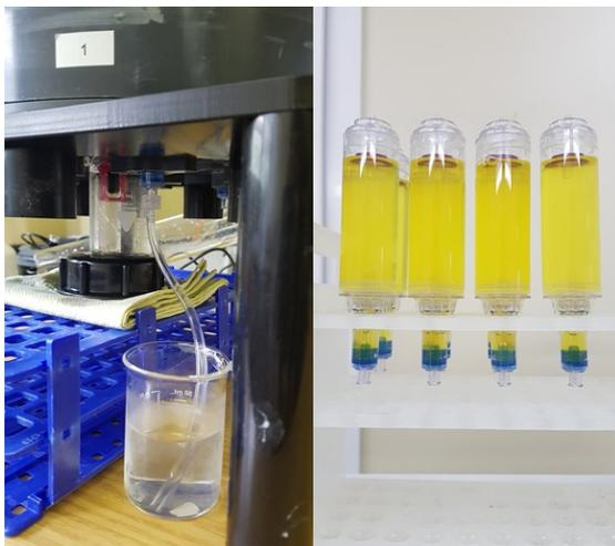
Figure 30: Left side: Sampling with cartridge 1 using a barb adapter with a tube. In the background: external temperature sensor. Right side: Filled sample cartridges after analysis.
