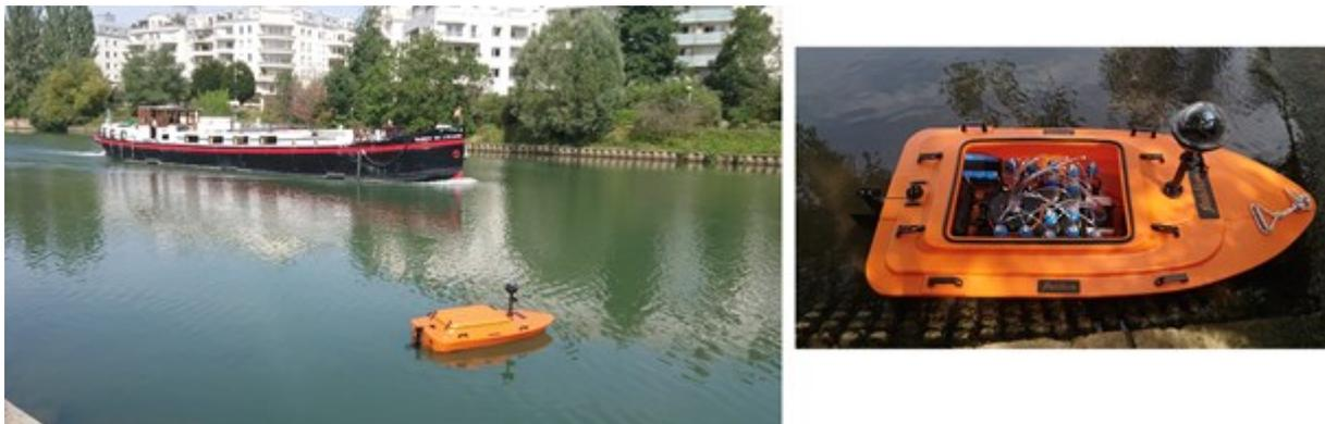
Figure 18: Fluidion DRONE usage for sample collection for performing spatial variability analysis in Marne river
