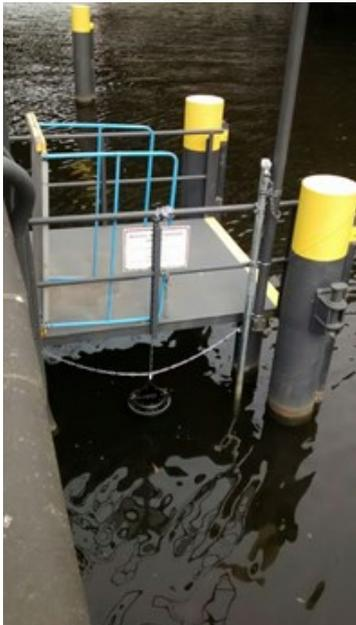
Figure 28: Fluidion ALERT System V1 installed in Spree-Canal for DWC campaign in 2019
