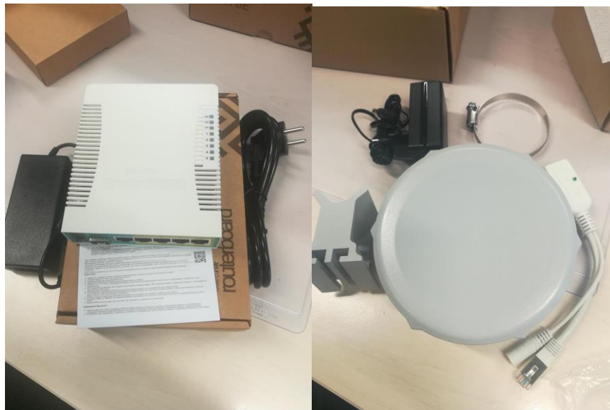
Figure 33. Mikrotik PoE and CPE with directional antenna Routers
