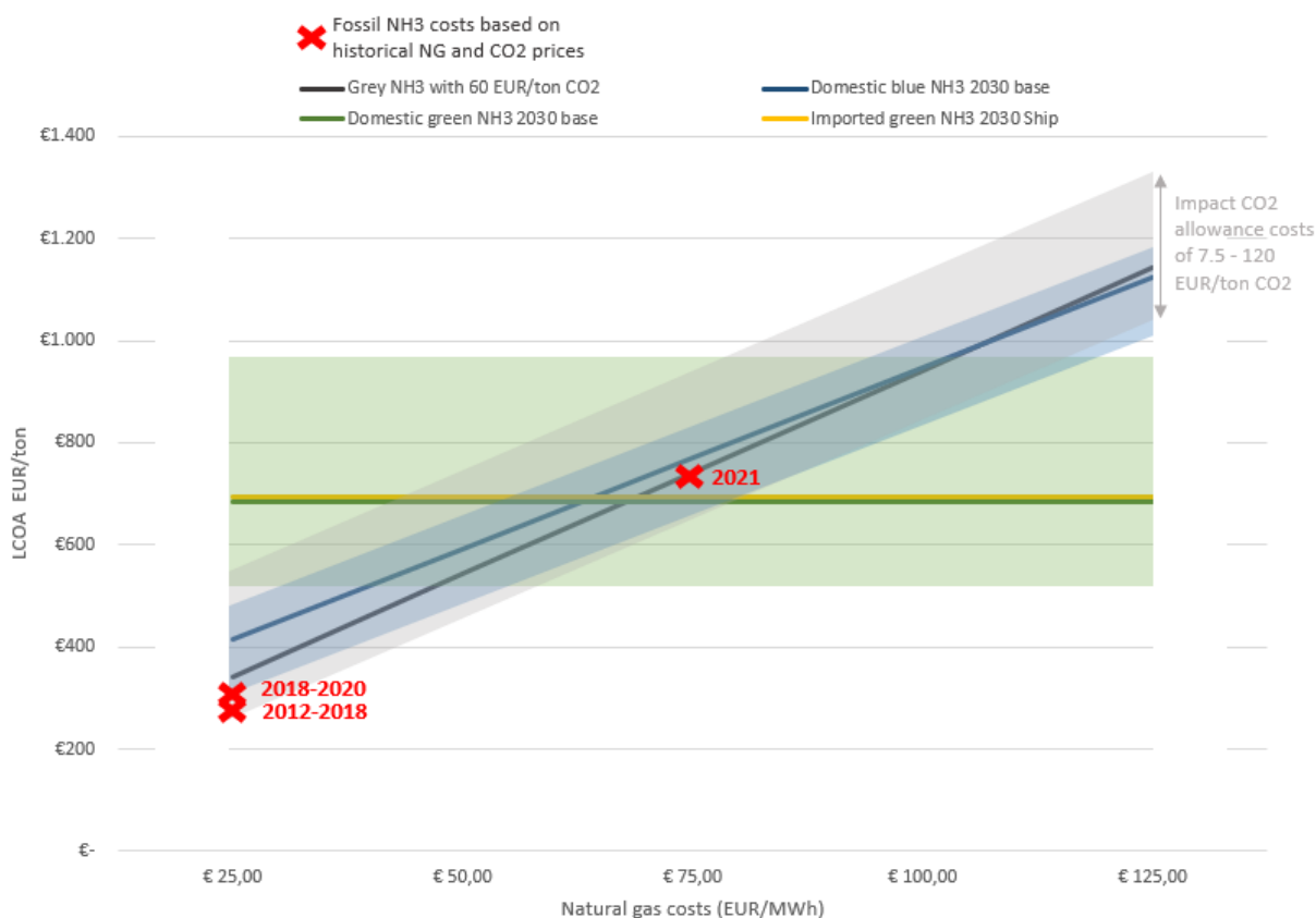
Figure 36 - Visualization of the impact of the natural gas and CO 2 prices on the reference price of NH 3 and on carbon-neutral NH 3 produced from blue hydrogen. The resp. green and blue areas mark the uncertainty cost ranges of the green and blue hydrogen production cost developments until 2030; the grey area represents the uncertainty in fossil NH 3 costs based on the CO 2 allowance price (7.5 EUR/ton low, 120 EUR/ton high). The levelized costs presented include transport to end-use site. The reference costs of NH 3 are calculated using 1.75-ton CO 2 /ton NH 3 [1], the natural gas and CO 2 prices of the past decade have been, resp. some 25 EU/MWh and 5-15 EU/ton CO 2 [2] [3] [4]. However, in 2021 a sharp increase of both European natural gas and carbon emission allowance prices is seen (since the autumn of 2021 the natural gas price rose to 80-180 EUR/MWh and the allowance price to 60-90 EUR/ton CO 2 ).
