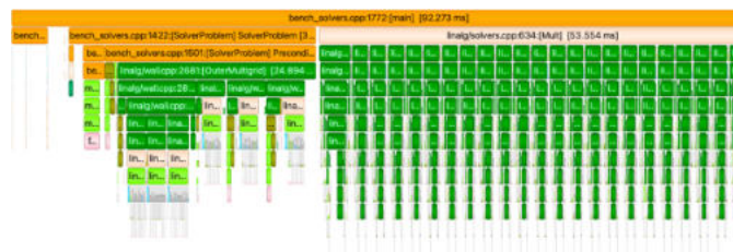
Figure 19: Intermediate steps can be introduced in order to allow graph optimizations of the kernel launches and the data movements. The best impact is when we are able to reduce the number of copies. This brings the benchmark time down to 54ms.
