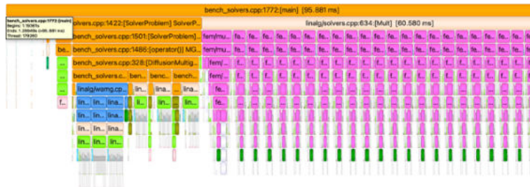
Figure 18: This step fuses the inner wavelet multigrid. Most of the software toolchain offline work is to prepare these transformations by populating the contexts which hold the needs of all the different kernels. This brings the benchmark time down to 61ms.
