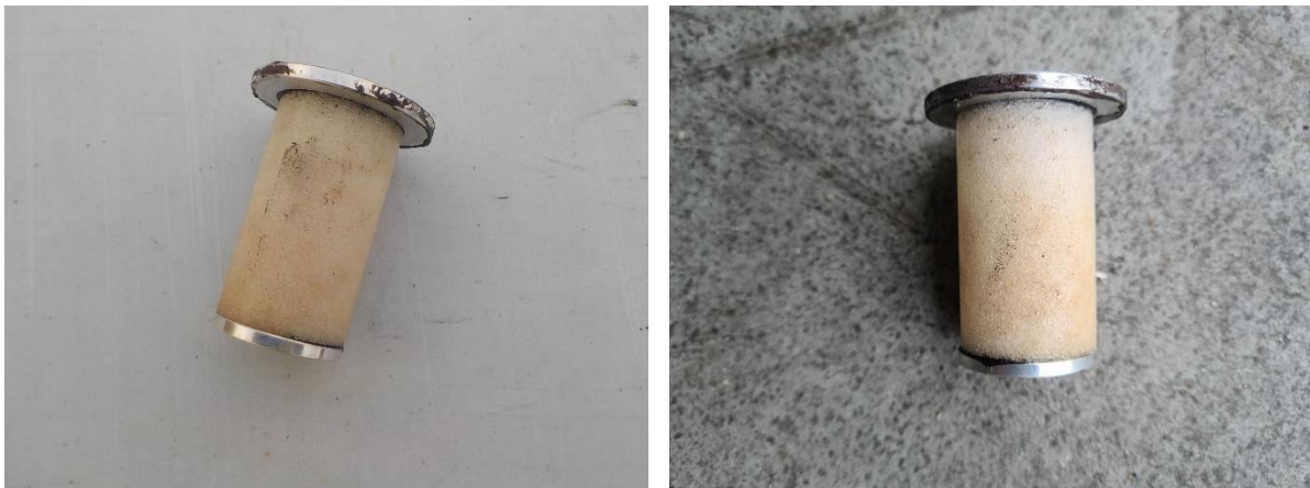
Figure 13: Gas filter before the start of the tests with natural gas (left) and after completion of the tests with hydrogen (right)
