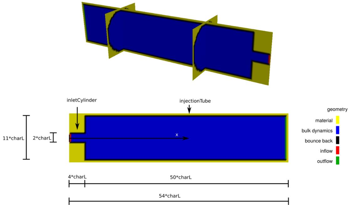
Figure 13.6: Cross section of a 3d geometry of nozzle3d in dependency of characteristic length  $charL$ .
