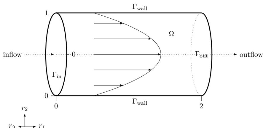
Figure 13.2: poiseuille3d geometry with boundary patches and velocity profile.
