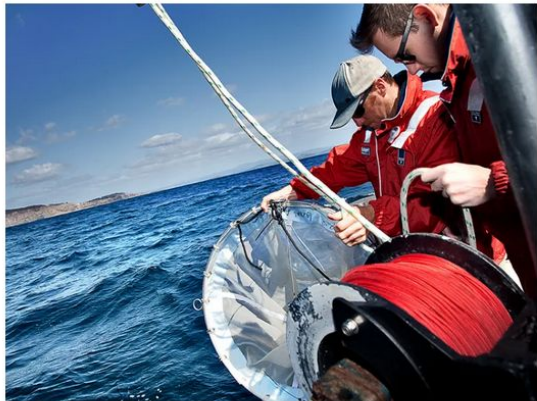
Plankton can be monitored in a variety of ways. Zooplankton diversity and biomass can be estimated by deploying collecting devices in the ocean, like the plankton net pictured here. Credit: Carlie Devine, CSIRO
