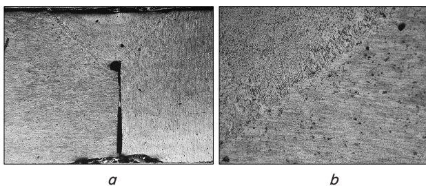
Fig. 8. Structures of laser-microplasma penetration: a – general view, \times 50 ; b – fusion zone with base metal, \times 250
