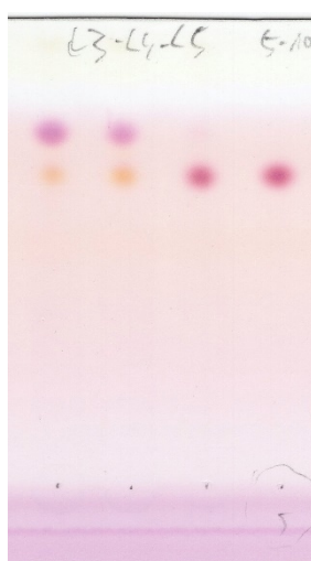
Figure 44: Chromatogram of 2 L. williamsii specimens containing no detectable mescaline (left), 1 specimen containing a low amount of mescaline (grafted L. williamsii on E. peruviana ) and a standard spot of mescaline on the far right for reference.
