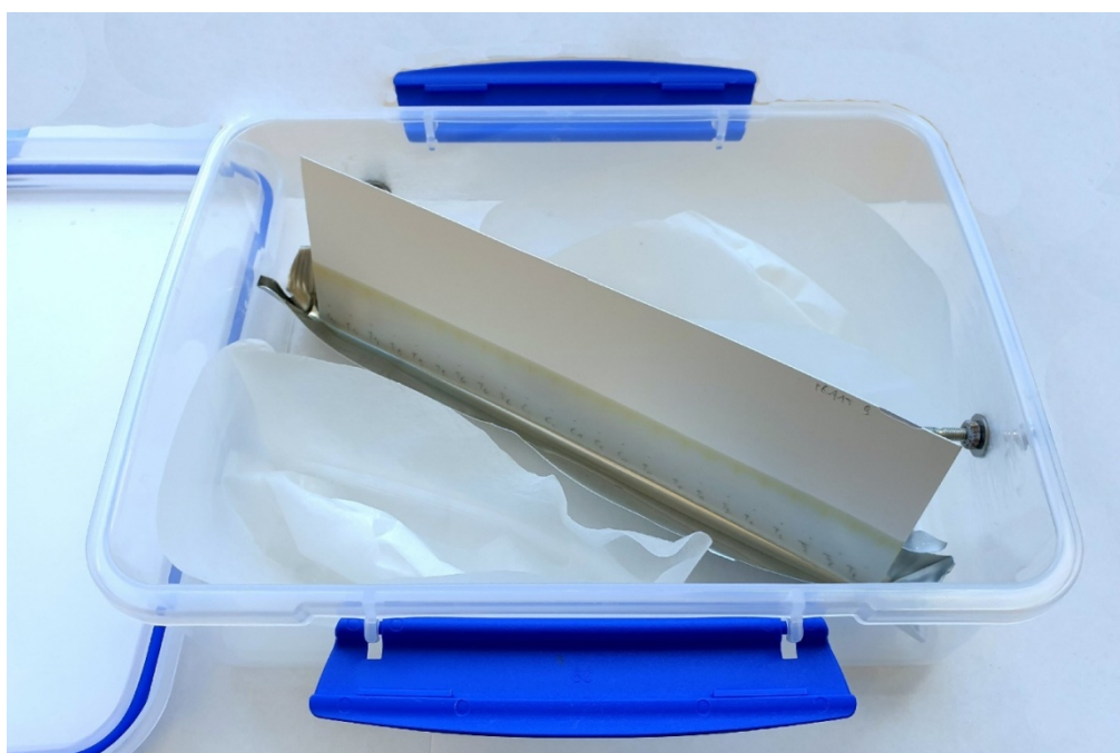
Figure 8: Development chamber made of polypropylene with aluminium holder for the plate and filter paper to saturate the chamber.
