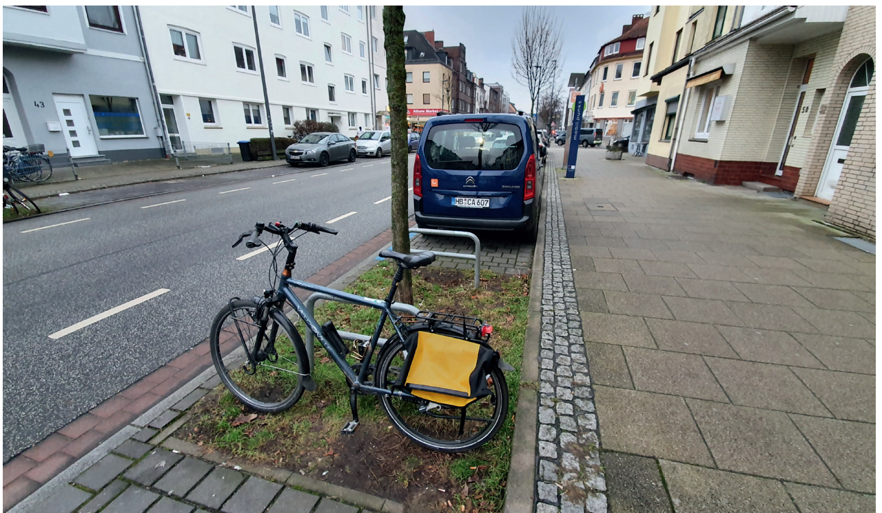
Figure 5: residential street in the City of Bremen – space competition for redesigned under climate resilience aspects – trees, safe walk and cycle conditions, unpaved strip for rainwater infiltration, Source: Glotz-Richter
