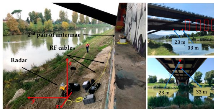
Figure 2.32. Experimental setup at the Varlungo Bridge in Florence, Italy (Miccinesi et al. 2021).
