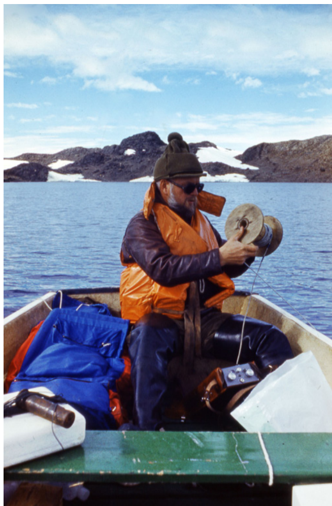
Enn Kaup profiling temperature and oxygen in Lake Algae in Bunger Hills (Antarctica), Photo: Enn Kaup
