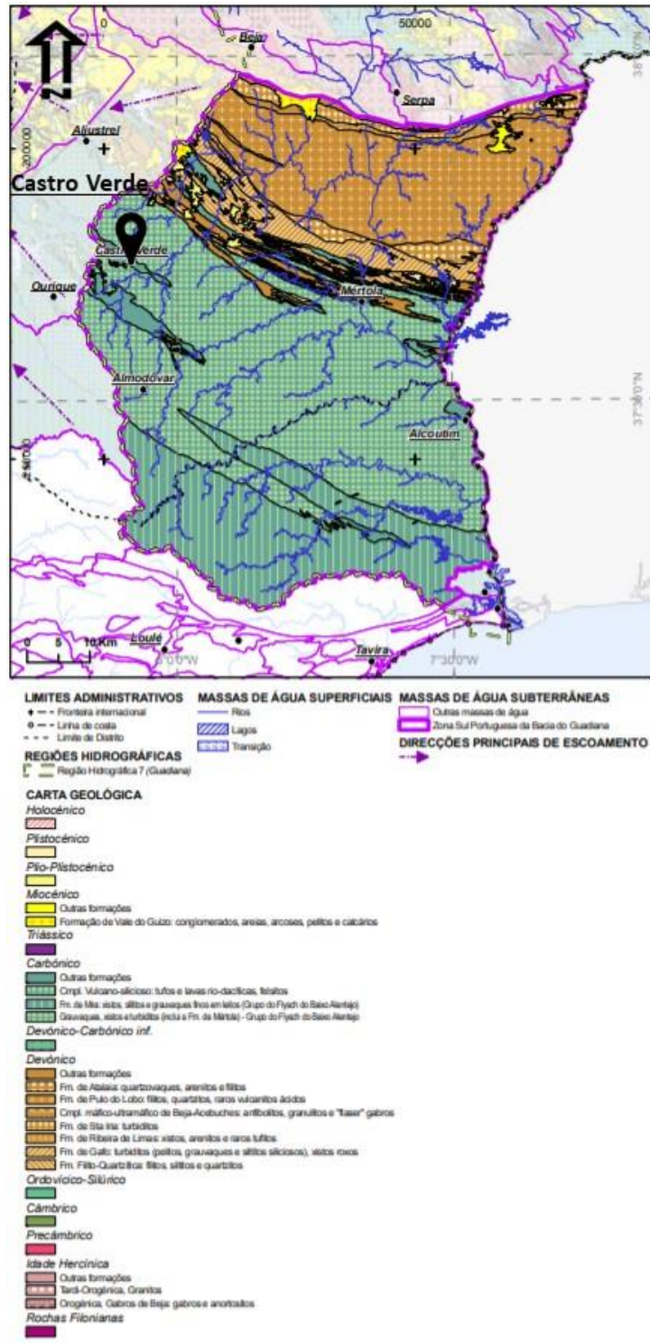
Figure 28. Geology of the groundwater body of the Portuguese South Zone of the Guadiana Basin (APA) [7]
