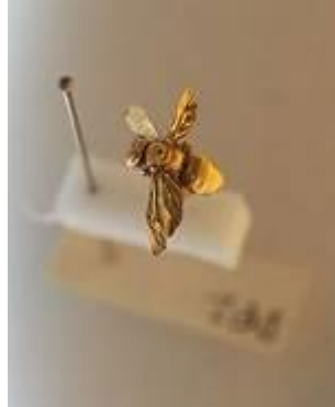
Fig.8: An insect coated in gold, having been prepared for viewing with a scanning electron microscope
