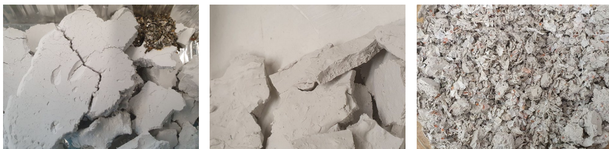
Figure 2.6: Solid reaction products after washing and filtration / drying. Left: S6 with unreacted metal impurities visible, middle: S8 from "pure" Al, and right: plastic impurities together with aluminium hydroxide in S4.
