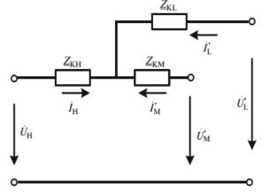
Fig. 1. Wiring diagram of the windings of a single-phase autotransformer.
