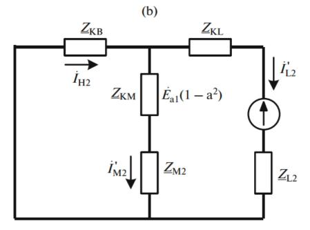
Fig. 6. Design schemes for (a) direct and (b) reverse sequence currents.  $\dot{I}_{H1} = \frac{\dot{U}_H - \dot{E}_{\alpha 1}(1 - \alpha) - \dot{I}'_{L1}(Z_{KL} + Z_{L1})}{Z_{KH}},$
