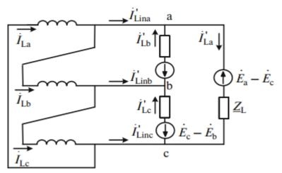
Fig. 5. Simulation of disconnecting the line wire on the LV side.
