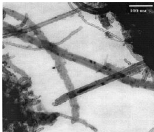
Figure 5. Micro-image of pyrolysis product of methane on cat №2 catalyst (temperature 560 °C, catalyst mass 10 mg, methane linear velocity 35 cm /min)
