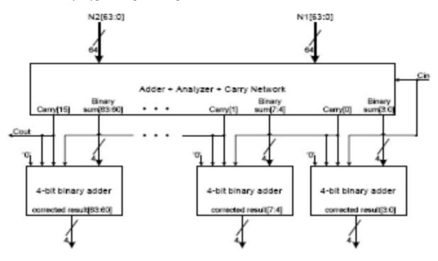
Correction is done by adding 0, 1, 6, or 7 to the binary sum coming from the first level adder. For each digit, the existence of the output carry and the input carry determine the value to be added for correction.
