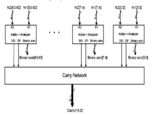
In our design, the DG and DP signals of a digit are computed as shown in the diagram. Equation 1 may simply find the output carries for each digit after having all the DG and DP signals. Input Carry=DG+DP Output Carry=DG+DP (1) We can generate DP by ANDing only
