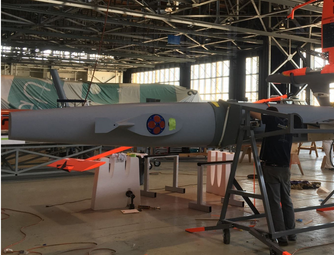
Figure 14. ADCP installed on a Saildrone (vehicle rotated 90 degrees to present the bottom of the hull).
