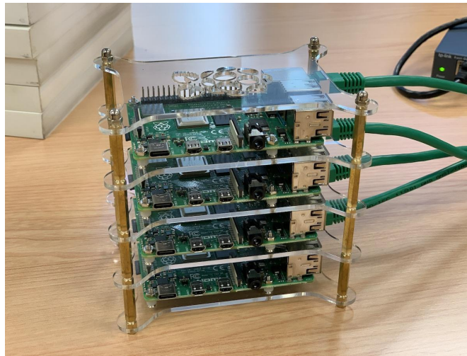
Figure 4.11 - Cluster of Raspberry Pis with four nodes to support OSCAR running on K3s for the edge.
