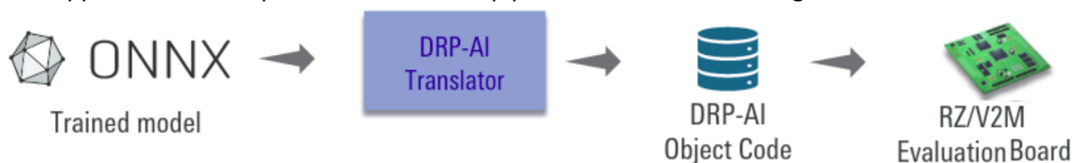
Figure 3.21 - RZ/V2M ONNX model import pipeline 104
