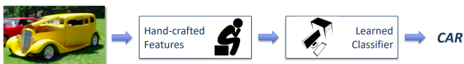
Figure 2.1 - Example of image classification with Machine Learning. Only the classifier is learned. Features are manually designed
