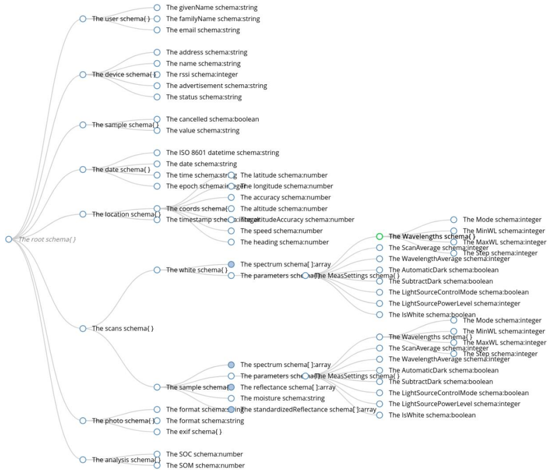
Figure 31: Quick graph overview of the schema used for the MEMS JSON data
