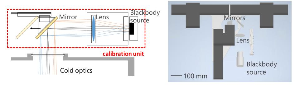
Schematic view of the on-board calibration unit (taken from Naruse-san's slide).
