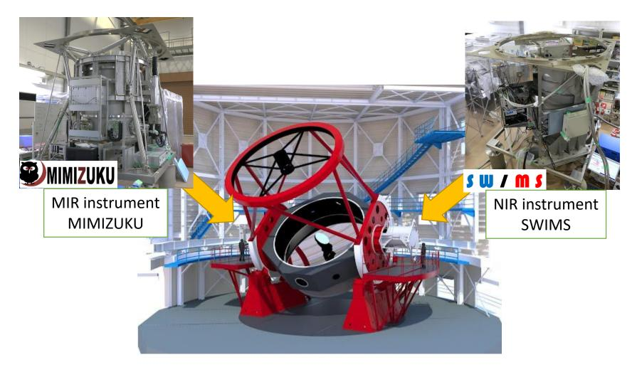
There are two first-generation instruments attached to the two Nasmyth foci.
