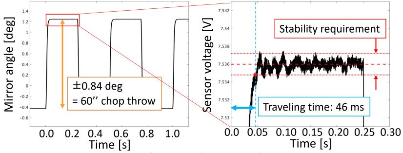
Chopper movement with a frequency of 2 Hz at 20 K (Michifuji-san's master thesis).
