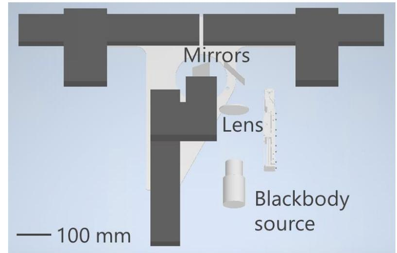
Schematic view of the on-board calibration unit (taken from Naruse-san's slide).
