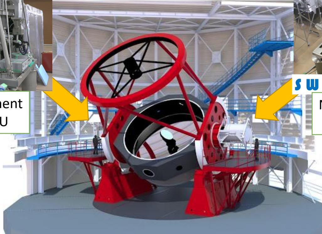
There are two first-generation instruments attached to the two Nasmyth foci.
