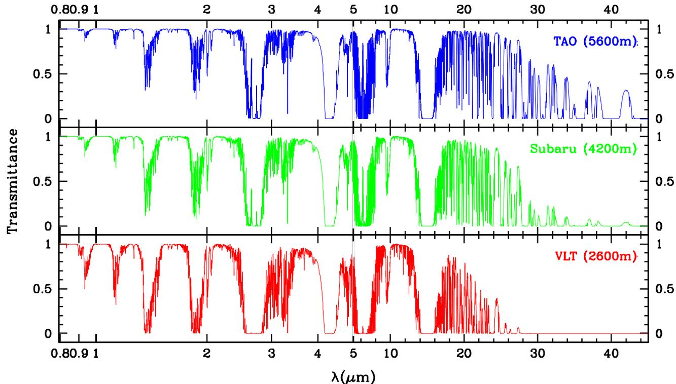
Atmospheric transmittance calculated by ATRAN.
