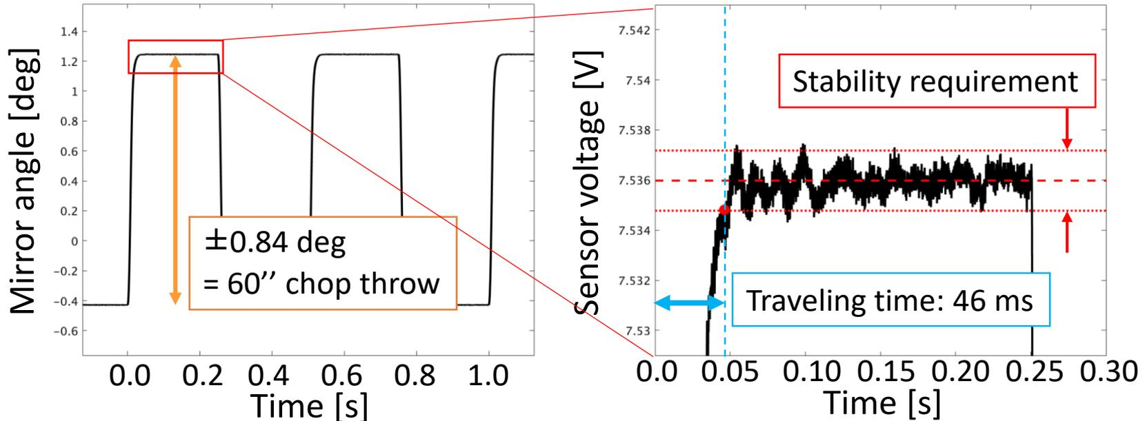
Chopper movement with a frequency of 2 Hz at 20 K (Michifuji-san's master thesis).
