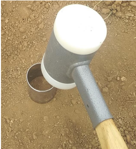
Figure 30: Undisturbed sampling tube placement with the aid of hammer
