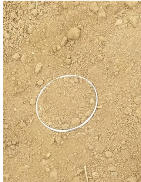
Figure 31: Undisturbed sampling tube marginally concealed to the ground
