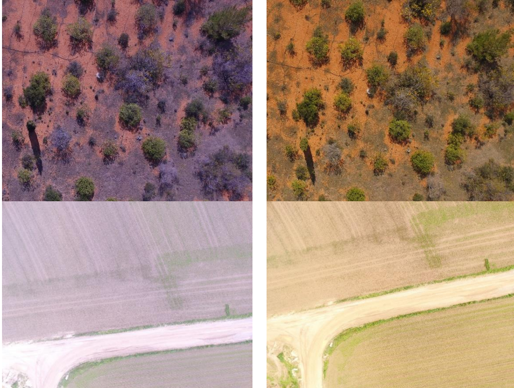
Figure 21: Left-side images indicate the false definition of the white balance effect; Right-side images are the colour corrected image after the conduction of the histogram matching approach.
