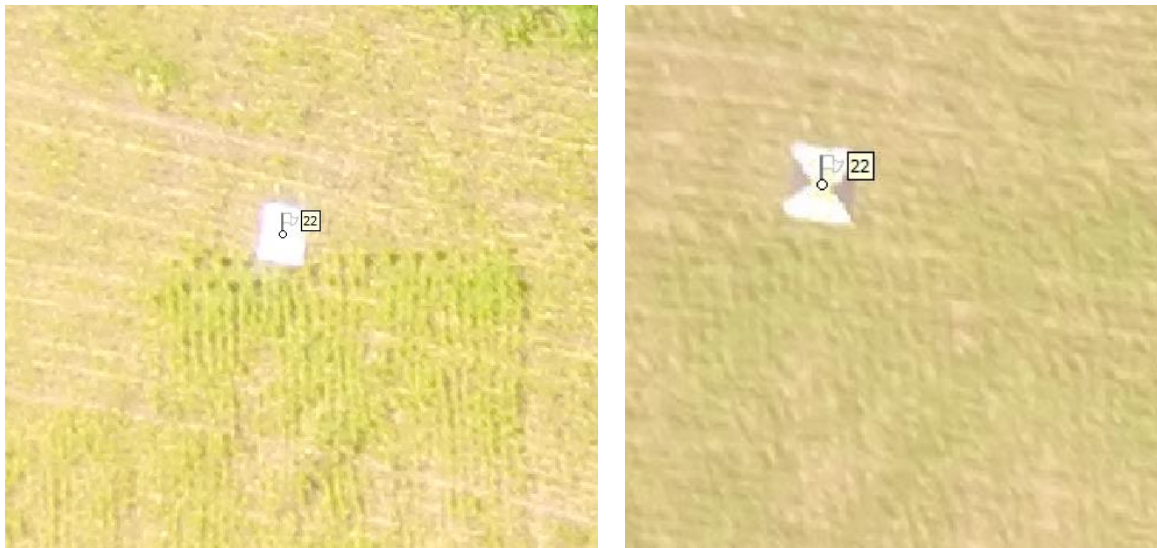
Figure 23: The left image presents a case in one of the Lithuanian drone flight campaigns, in which the markers cannot be used in the calibration process of the image orthomosaic as the center of the marker is not visible and the collected GCP cannot be placed correctly. The right image presents a photo over the same case where the marker can be recognised.
