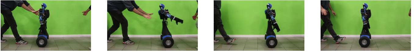
Fig. 2: Experiment - Dynamic disturbance . When an external disturbance is applied, the robot arms motion contributes visibly to stabilize the pitch angle
