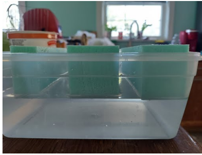
(b) Foam block floating in a water with density ratio of around 0.05.
