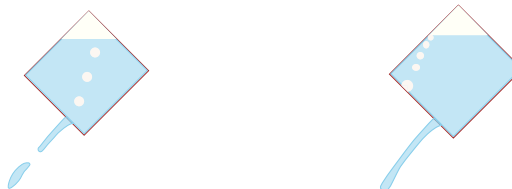
Fig. 16.11 – Counter-current flow in a can (the left figure) has only one hole thus pulse flow and a flow with two holes (right picture).
