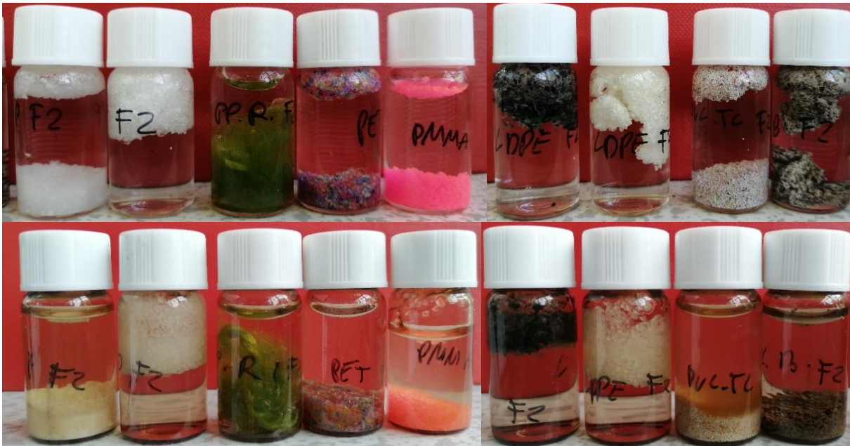
Fig 3: Five different types of MP from a range of sources in water. Top is before treatment with an electron beam, bottom is afterwards. Note that after treatment almost all the MPs are either floating or have sunk, hence providing routes for removal using standard techniques.
