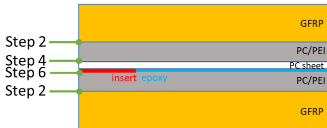
Figure 13. Bonding steps for AM specimens.
