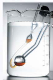
Fig 3. Capillary viscometer used in the study
