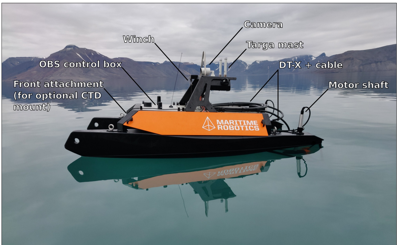
Figure 2: Otter USV in the field in Billefjorden . Parts of the DT-X and its cable were located in the rear (right). The camera as well as the various radio/wifi antennae are mounted to the top of the USV's OBS control box on the left.
