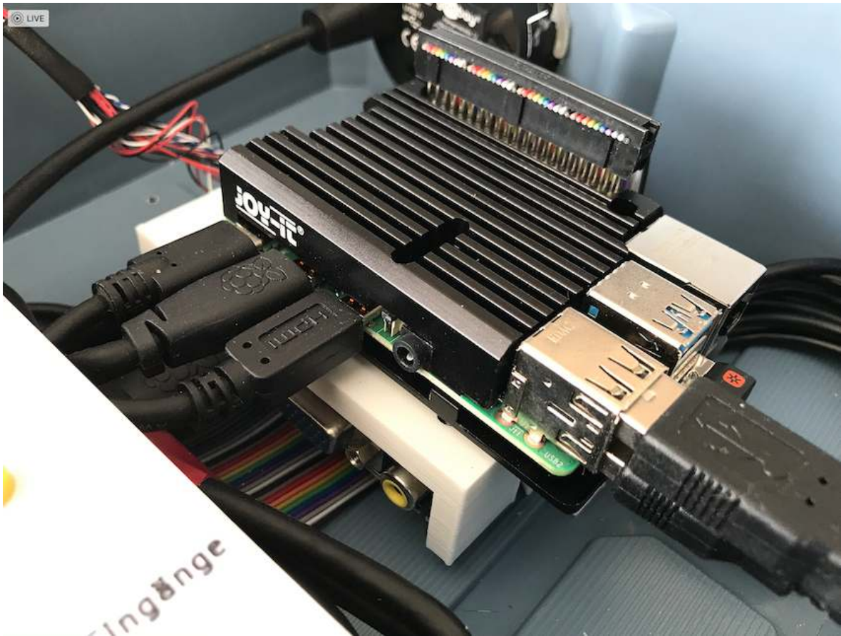
Fig. 18: Case construction, step 10: Attach the display controller housing to the case
