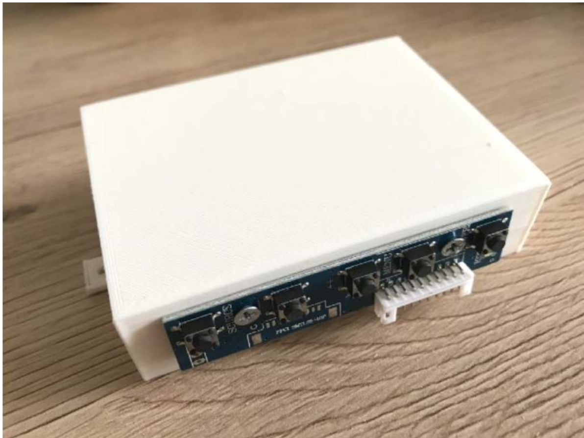
Fig. 14: Case construction, step 8: Screw on the display controller
