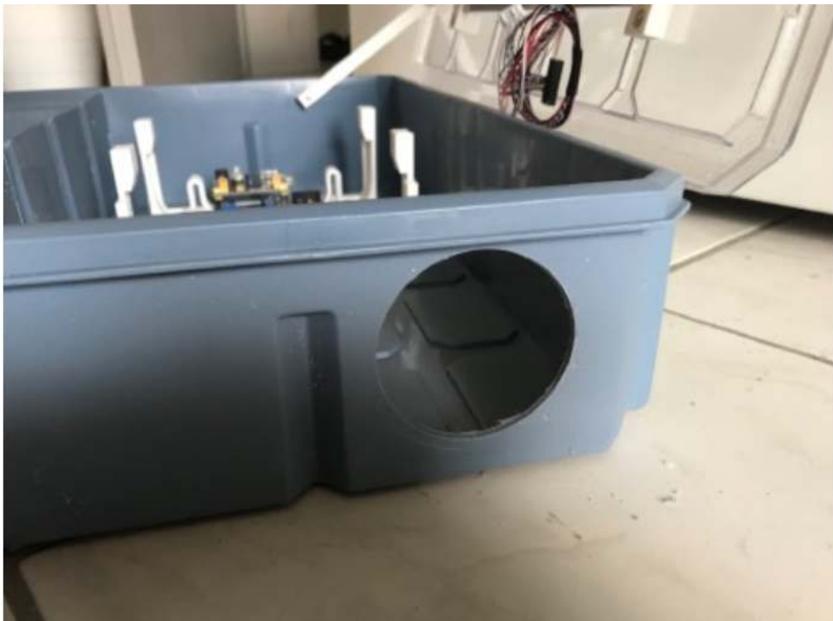
Fig. 12: Case construction, step 6: Drill a hole for the USB hub
