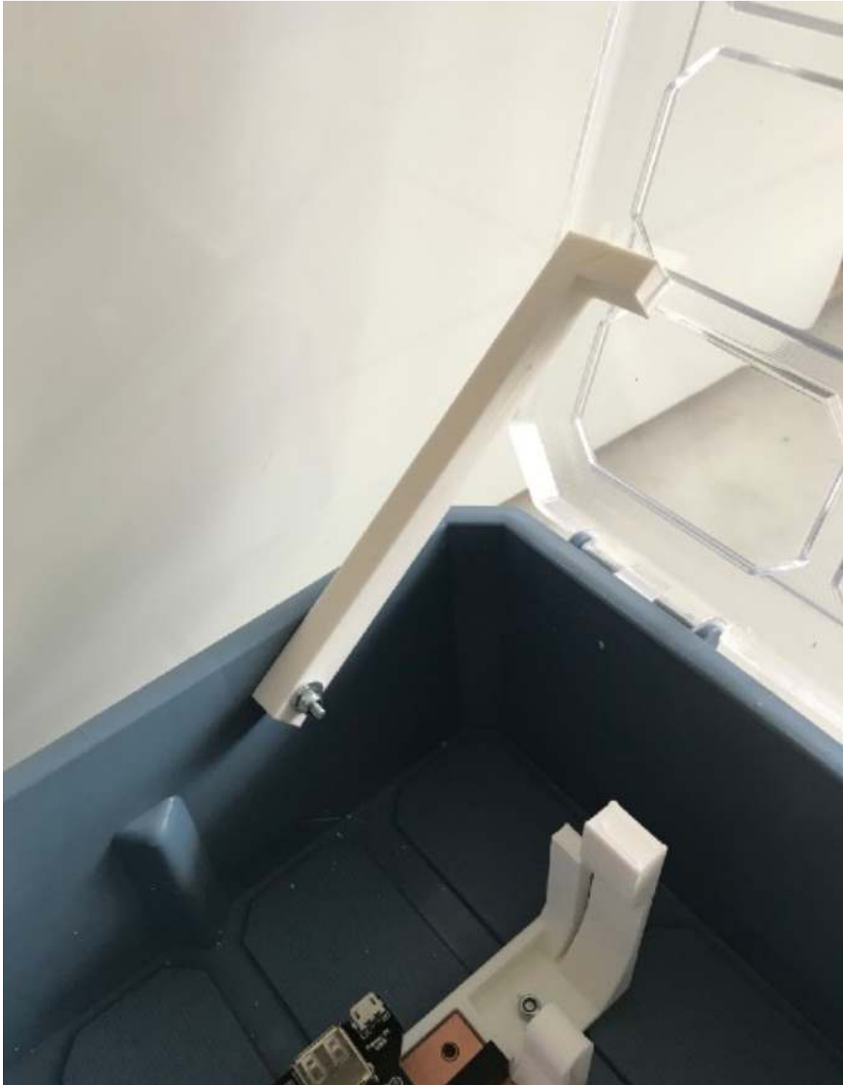
Fig. 10: Box construction, step 4: screw on the retaining rod
