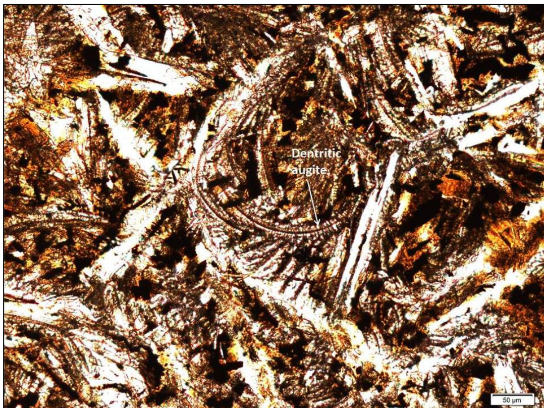
Figure S 3-3. Augite that has crystallized fast in a cool environment commonly becomes dendritic. Here exhibiting curved, branching dendrites. View in PPL.
