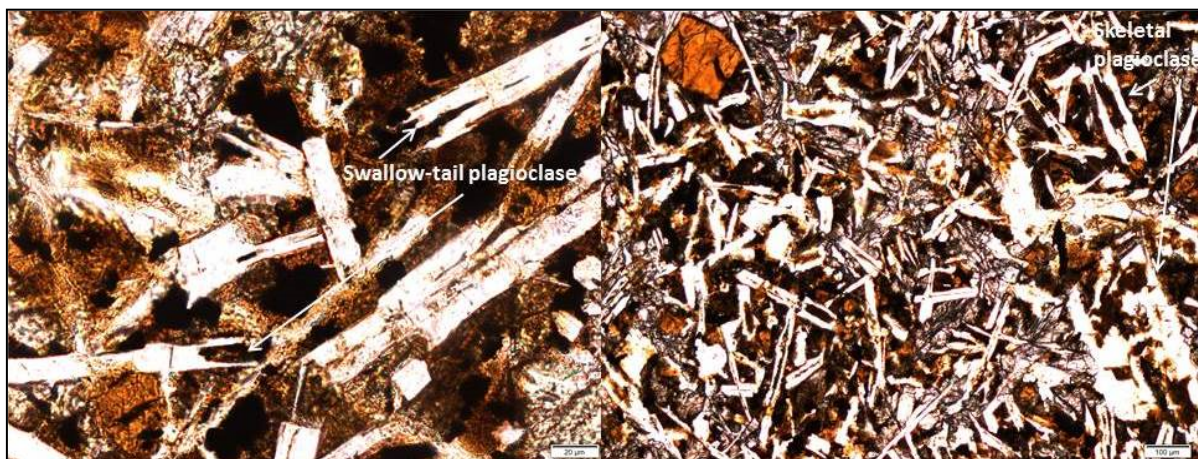
Figure S 3-1. Plagioclase exhibiting swallow-tail morphology and skeletal growth. View in PPL.
