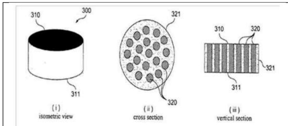
**Fig. 3:** Schematic Diagram of Innowattech Piezo Electric Generator.
