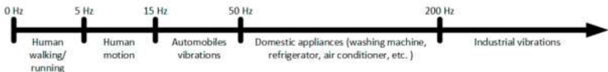
*Fig. 1: Different Mechanical Energy Sources – Frequencies.*
